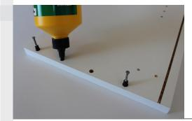
Proceed to insert the metal dowels into the outer two holes on the side panels at both ends.
