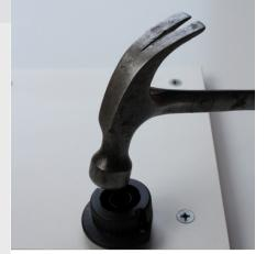
The leg sockets are inserted in to the remaining holes on the underside of the base panel. Twist in and ensure that the flat side of the socket is aligned to the front of the cabinet, leaving the curved edge facing the back. Use a hammer to gently tap in.
