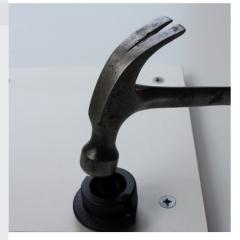
The leg sockets are inserted in to the remaining holes on the underside of the base panel.
