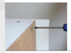
Insert the back panel into the grooves of the side panel. Fix into position using the roundhead screws provided, fixing the screws evenly spaced along the top and along the bottom of the panel into the top and the bottom panel.
