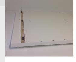
For the remaining half of the corner cuboards, repeat the process above, this time placing the dowels into the groove on one of the side panels as per image.
