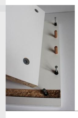
At this stage be sure that the white edges of the top and bottom panels are facing the front of the cabinet and proceed to tighten the cams with a cross head screw driver.
