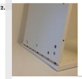
Proceed to insert the wooden dowels into the corresponding holes in the base panel. Again prior to inserting applying a small amount of wood PVA glue into the holes.
