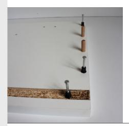
On the top and botton edge of the side panel, insert a further two metal dowels into the two outside holes and two wooden dowels into the inner holes. Again when inserting the dowels apply a small amount of PVA glue into the holes.
