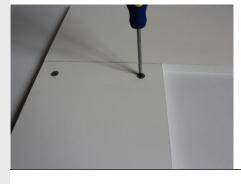
To assemble the shelves take one large and one small sized shelf piece. Insert two metal dowels into the pre cut holes in the larger of the two shelf pieces.
