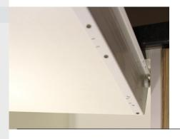
Make up the drawer, as per image, using again the cross head screw driver and six screws per side; four on the underside and two on the back.
