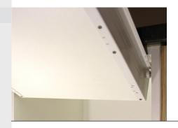
Make up the drawer, as per image, using again the cross head screw driver and six screws per side; four on the underside and two in the back.
