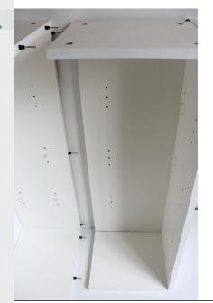
The larger and small cabinets can now be fixed together. Insert the metal dowels into the holes on the larger cabinet, as shown and insert into the corresponding holes on the smaller of the two cabinets.
