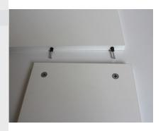
To assemble the shelves take one large and one small sized shelf piece. Insert two metal dowels into the pre cut holes in the larger of the two shelf pieces. Connect the two pieces together as per diagram and finish by tightening the cams.
