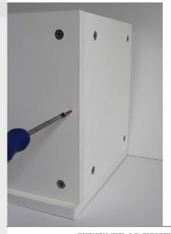
To finish fixing the side panel into position fix three 30mm screws along the top and bottom edges of the panel.
