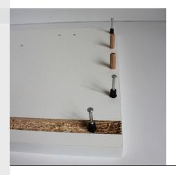
On the top edge of the side panel, insert a further two metal dowels into the two outside holes and two wooden dowels into the inner holes.
