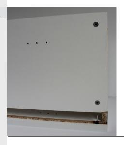
Once the top and bottom panels are fixed in position take the remaining side panel and insert into the pre cut groove, making sure again at this stage that the white edge is facing the front of the cabinet. Proceed to tighten the cams with a cross head screw driver.
