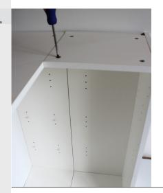
Again proceed to tighten the cams with a cross head screw driver.
