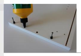
Proceed to insert the metal dowels into the outer two holes on the side panels at both ends.
