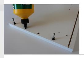
Proceed to insert the metal dowels into the outer two holes on the side panels at both ends. 3.
