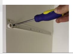
Using a cross head screw driver fix the drawer runners into position according to the pre drilled holes provided using five screwa for each runner.
