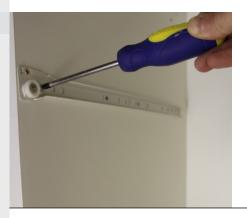
Using a cross head screw driver fix the drawer runners into position according to the pre drilled holes provided using five screws for each runner.
