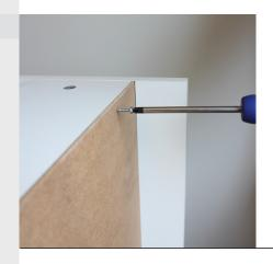
Insert the back panel into the grooves of the side panel. Fix into position using the roundhead screws provided, fixing 3 screws evenly spaced along the top and along the bottom of the panel into the top rail and the bottom panel.
